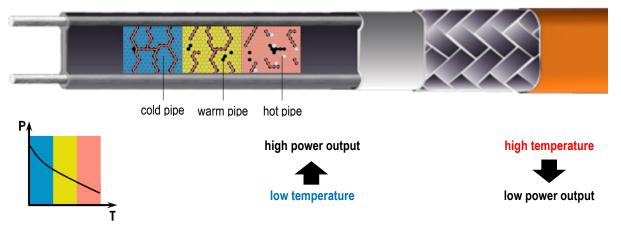
The trace heaters are fixed equipment heating systems for pipes in ordinary and hazardous / industrial areas. Thanks to the parallel design the trace heater can be cut and installed to any required length (up to the maximum heating circuit length as shown the BARTEC Design Guide).
