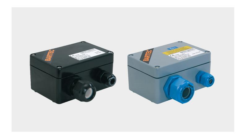
The junction boxes for Pt100 Ex allow one or more two-wire or three-wire Pt100 resistance thermometers to be connected to the signal line.
